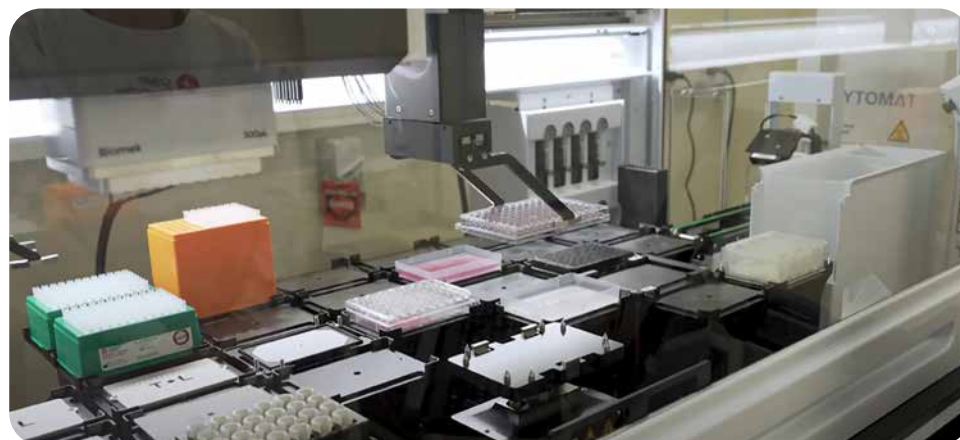
The robotic arm speeds up the work with samples.
